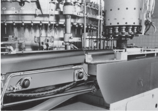
Bottle filling line conveyor
