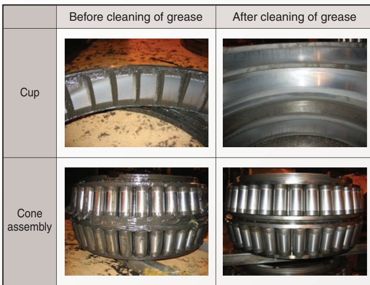
Post-use appearance of bearing with high-performance seal
