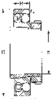
Tapered Bore Taper 1:12 on Dia.
