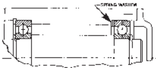
Mounting with Snap-Rings and Spring Washer
