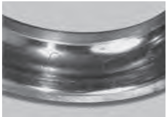
Fig. 15-8 Indentation and Flaking on Outer Ring Raceway of Deep Groove Ball Bearing
