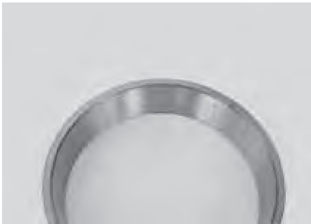
Fig. 15-7 Indentation Marks on Outer Ring Raceway of Tapered Roller Bearing
