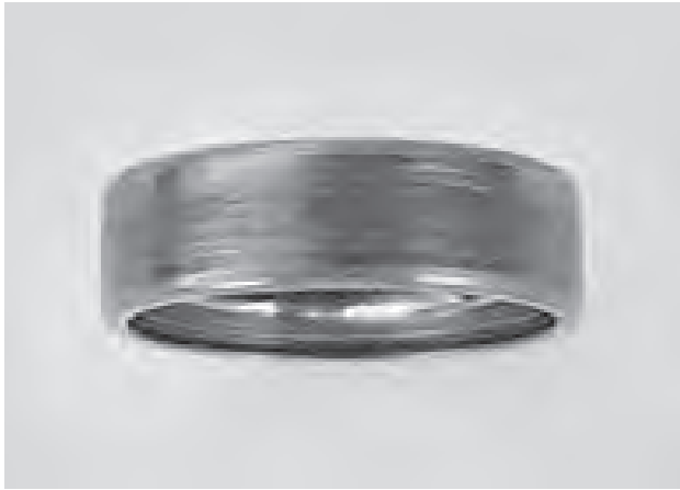
Fig. 15-9 Creep on Outer Ring Surface of Deep Groove Ball Bearing
